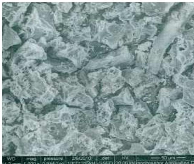
Figure 3 : Morphology of BaFe<sub>12</sub>O<sub>19</sub> nanomaterials, annealed at 750°C
