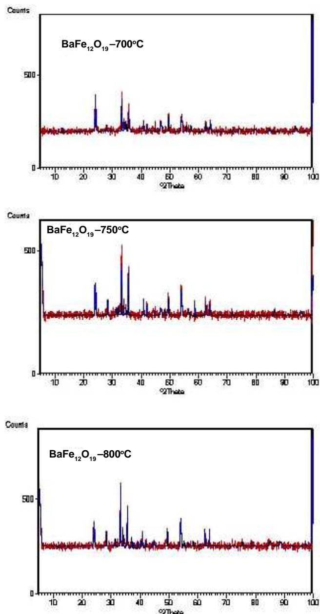
Figure 1 : Xray Diffraction Patterns for BaFe<sub>12</sub>O<sub>19</sub> Nanoparticles annealed at temperature 700°C, 750°C and 800°C
