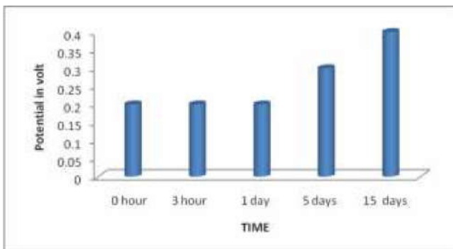
Fig. 4. Graph showing variation in potential difference generation with time period with Ananas comosus as substrate
