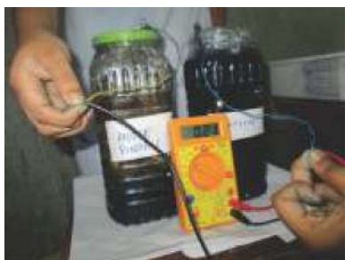
Fig. 11. Figure showing Microbial Fuel Cell set up made using Ananus comosus as a substrate
