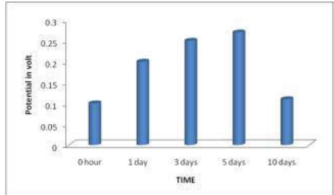
Fig. 7. Graph showing variation in potential difference generation with time period with mixed sample as substrate
