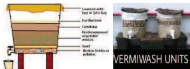
VERMIWASH UNIT: DIAGRAMMATIC
