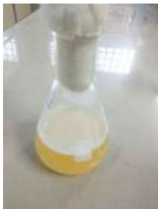
Fig. 1. Top layer indicating the presence of bio surfactant after 7 days of incubation
